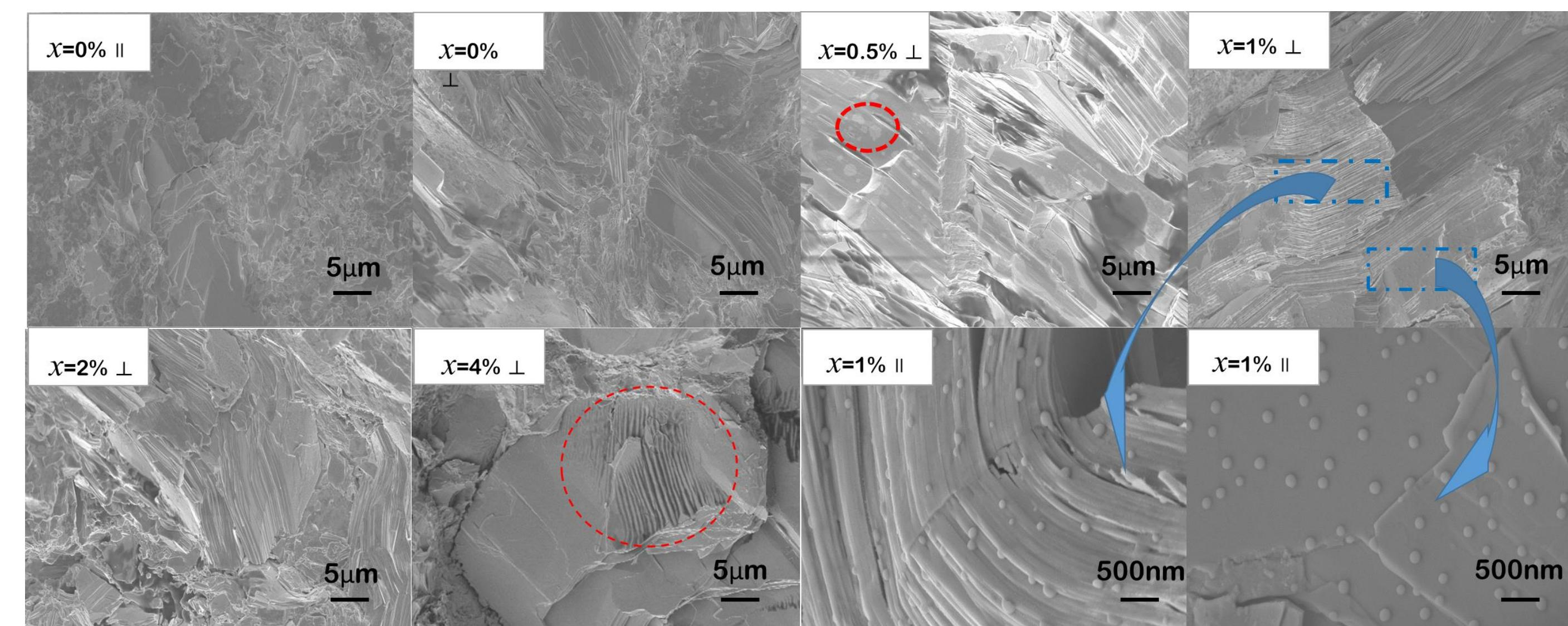
SEM: microstructure variable with the amount of MoSe<sub>2</sub> specially in  $\perp$  direction
